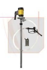
Each package comes complete with an electric motor, 39" (1 m) pump tube, dispensing nozzle, 6' (1.8 m) of chemically resistant hose, barrel adapter, pump storage bracket and hose clamps.
